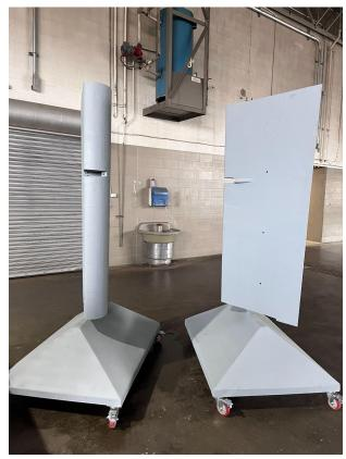
The wing is coated with an enamel primer. The use of an acrylic based paint to apply the final rendering and seal with a water-based polyurethane is recommended.
